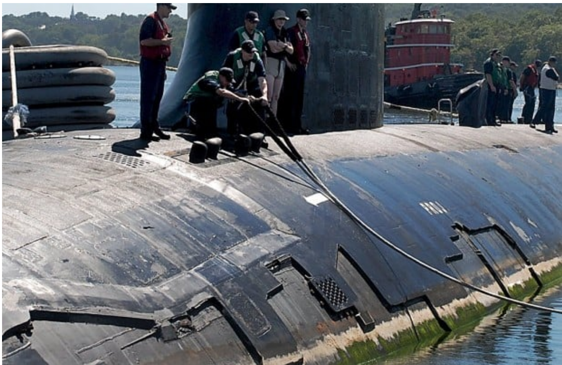
Figure 25: Missing tiles on a Virginia submarine (Creator: MC2 Jonathan Sunderman | Credit: U.S. Navy)
